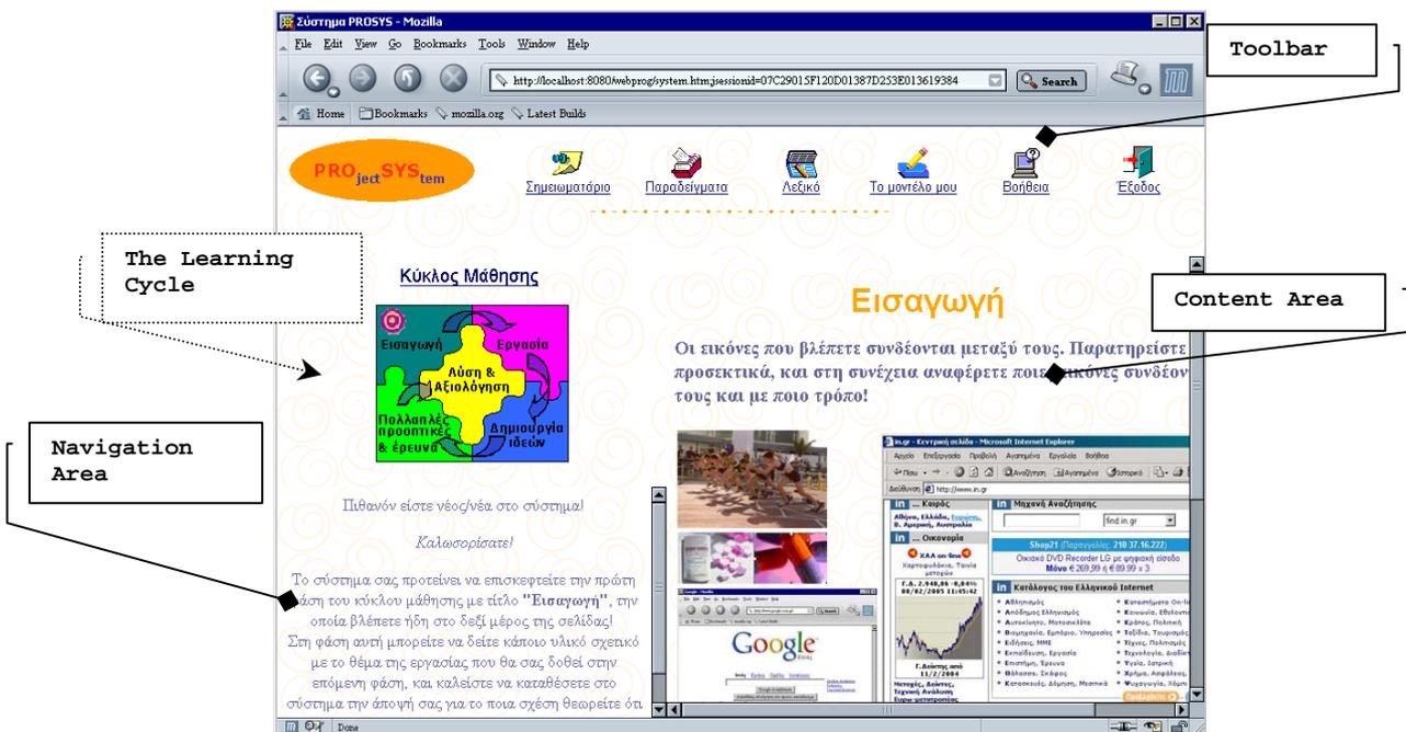
Fig. 1: The main screen of ProSys consists of (a) Toolbar (b) Navigation area on the left including the Learning Cycle (c) Content area on the right that presents instructions, activities, content at each stage
